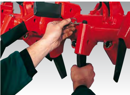
CULTITILLER FAST-FIT®: A KUHN exclusive, fitted with only one lynch pin, tines are replaced within minutes and their hold is not affected.
