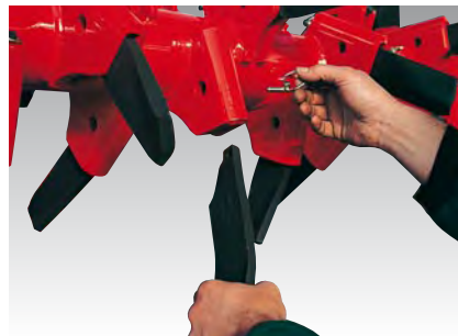
CULTITILLER FAST-FIT®: A KUHN exclusive, fitted with only one lynch pin, tines are replaced within minutes and their hold is not affected.
